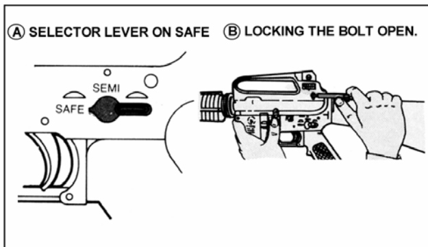
Figure 5-33. Clearing an M16A2 rifle.
